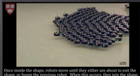
Once inside the shape, robots move until they either are about to exit the shape, or bump the previous robot. When this occurs, they join the shape.
